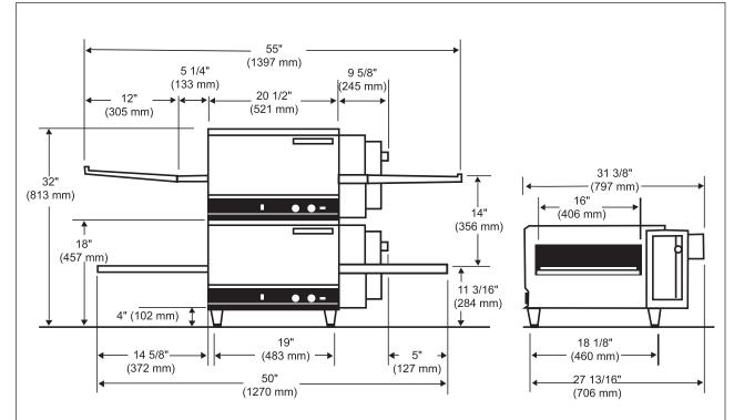
**ELECTRICAL SERVICE**: Heat is supplied by one (1) element at 5600 watts. Each oven is rated at 6kW. The ovens are available in 208V and 240V and are single phase. The oven comes with a factory installed cord wth NEMA 6-50 plug. A separate circuit breaker is required for each oven deck with the proper voltage, amperage, phase and hertz as indicated by model number.
